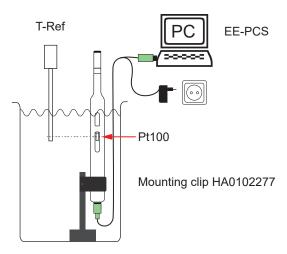
Fig. 7 Temperature calibration/adjustment in a liquid bath
