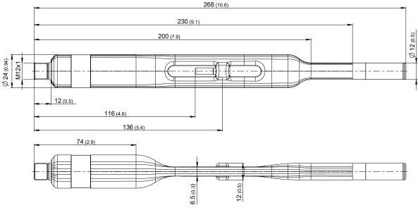
Fig. 1 Dimensions of EE260 in mm (inch)
