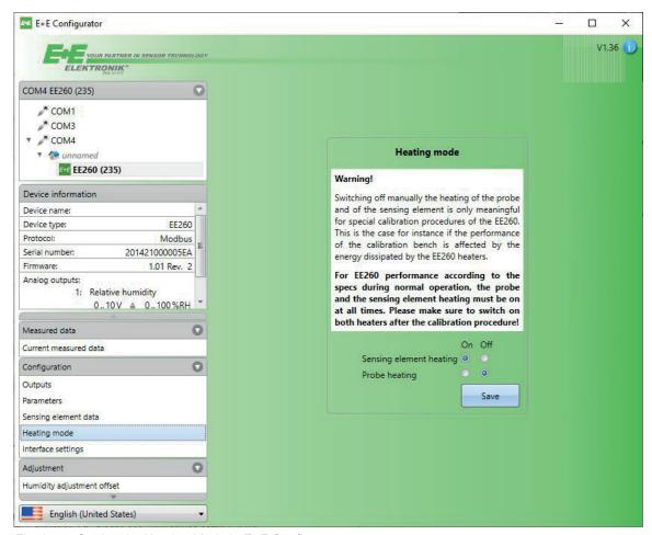
Fig. 6 Setting the Heating Mode in E+E Configurator
